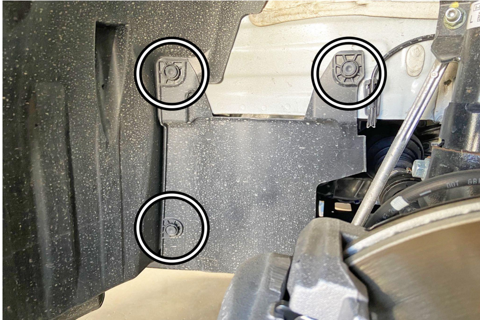
7. Remove the three retaining clips.
