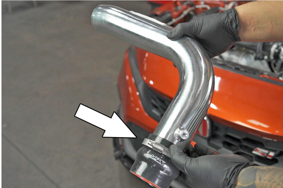
19. Secure the hump coupler along with the provided clamp onto the HPS intake pipe.
