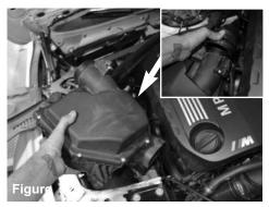
Pull back the intake hose, now lift up and remove the passenger side air box out of vehicle.
