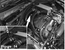
Loosen clamps on the top of the intercooler.
