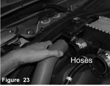
Position the machined fitting to the turbo, and the pipe to the straight hose
