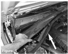
Loosen the engine tray and pull back weather trim
