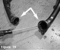
Using a flat head screwdriver, remove the o-ring gaskets from the stock charge pipes.
