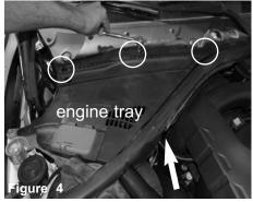
Loosen the 3 plastic screw fittings holding in the engine tray connected at rain gutter.
