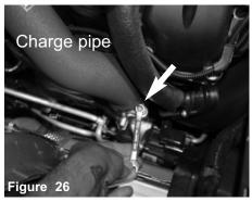
Secure the charge pipe using oem bolt from step 17. Secure and tighten using 8mm wrench.
