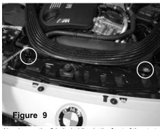
Now loosen the 2 bolts holding in the front of the strut bar on the radiator support.
