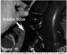
Loosen the bolt holding in the intake tube using 10mm socket and ratchet.
