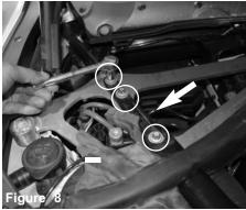
Loosen the 3 bolts on the end of the strut bar and remove. Continue on other side.
