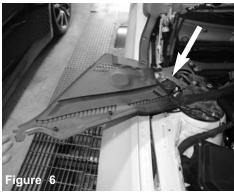
Lift up and turn the engine tray out of the way. This will Loosen the 10mm bolt holding the strut bar on allow for removal of the factory strut bar. Now repeat and do on other side of vehicle.
