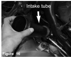
Now remove the intake tube from vehicle.
