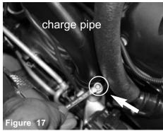
Loosen the bolt holding in the Lower part of the charge pipe to the turbo using 8mm wrench.Save bolts for re-install. *Repeat on the other charge pipe*.
