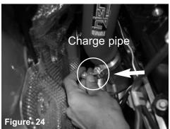
Secure the charge pipe using oem bolt from step 17. Secure and tighten using 8mm wrench.
