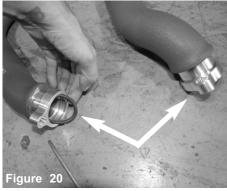
Now install the o-ring gaskets to the inside of the injen charge pipes.
