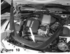
Now lift up and remove the factory strut bar. This will now have access for the intake systems.
