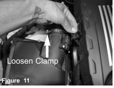
Disconnect passenger side MAF sensor harness. Loosen clamp on air box.
