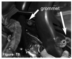
Lift up and pull charge pipe out of the grommet. Lift up and remove from vehicle. *Repeat on the other charge pipe.*
