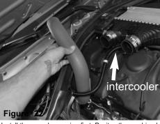
Install the rear charge pipe first. Positon the machined fitting to the turbo, and the pipe to the straight hose.
