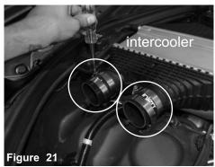
Install the 2-1/4" straight hose with clamps to the intercooler. Tighten the clamps on the intercooler only.
