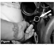
Loosen the clamp on the turbo housing using 7mm nut driver. Now lift up and remove passenger side intake tube from vehicle.
