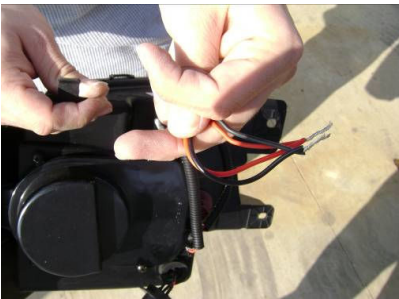
Step 12: Twist the two red wires together and the two black wire together from the Anzo headlight assembly.
