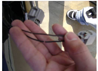
Step 13: locate the side maker light, pull back the electric tape exposing the black and brown wire on the stock harness.
