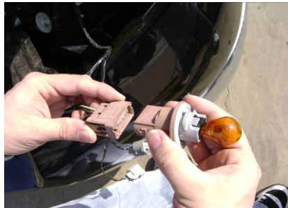
Step 10: Disconnect the inner signal bulb socket from the wire harness.
