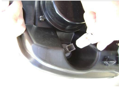
Step 16: Plug the side marker harness to the socket.
