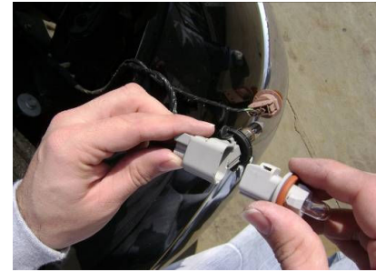
Step 11: Disconnect the side marker socket from the wire harness.
