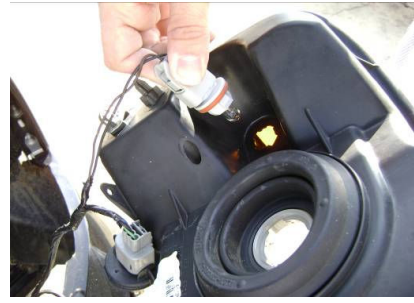
Step 8: Twist and pull the side maker light out of the headlight housing.
