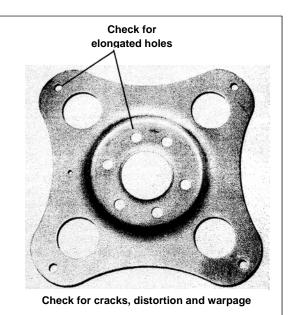
14. Check the bolt pattern on your B&M torque converter and make sure it matches your flexplate.
