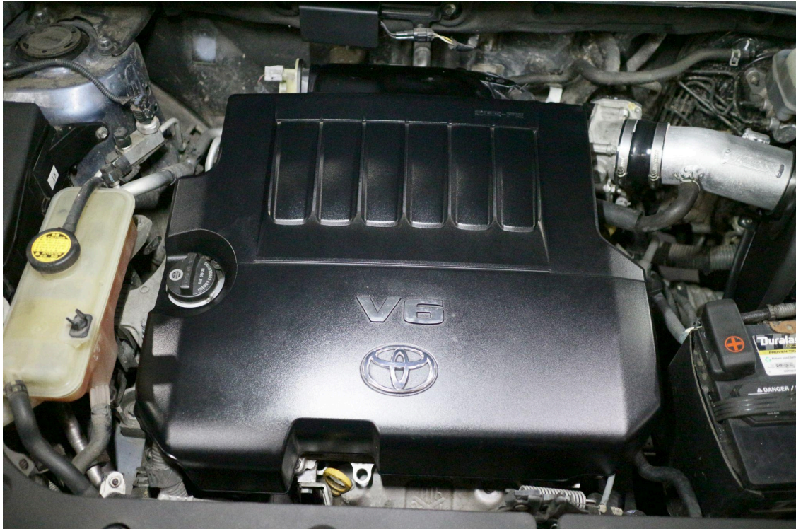
35. Reinstall the plastic engine cover.
