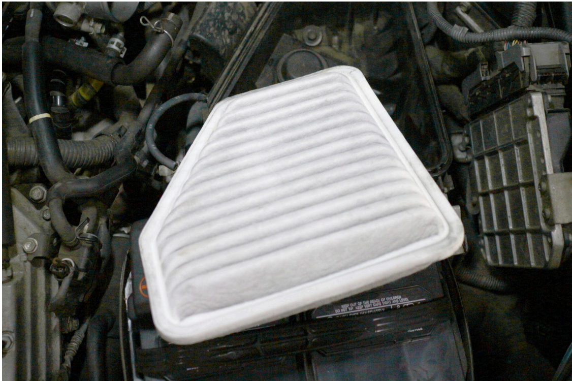
15. Remove the air filter from the lower air box.
