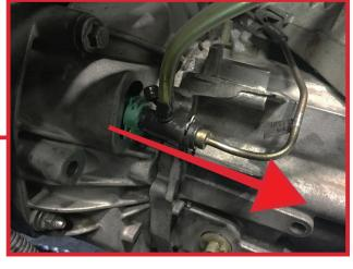
Fill the reservoir with fluid and allow the fluid to gravity bleed. Once fluid is flowing, use your hand to slowly depress the pedal by <sup>3</sup>/<sub>4</sub> stroke and back checking the reservoir level. Continue until no more air bubbles are flowing.
