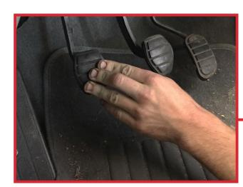
Once the air is out of the system. Push the hard line in fully to seal the bleeder port and check the clutch pedal has a normal operation.
