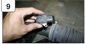
Remove MAF sensor using phillips screwdriver.
