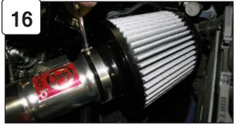
Attach air filter to tube and tighten using 5/16" nut driver.
