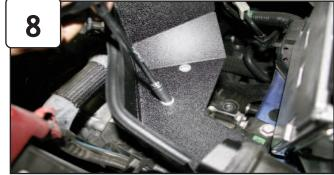
Install housing into vehicle and position. Secure hous-ing using provided M6 screws and flat washers. Tighten using 10mm socket or wrench.
