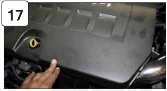
Re-install engine cover. Re-connect battery terminals.
