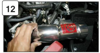
Install intake assembly and position. Do not tighten.
