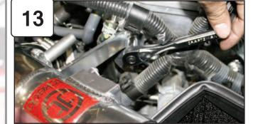
Secure tab on tube to engine. Re-install bolt from step 11 and tighten.
