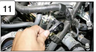
Loosen bolt on side of engine using 13mm socket or wrench.
