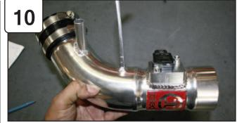
With provided M4 screws, install MAF sensor to new intake tube. Attach 05-00570 coupler with clamps to tube.
