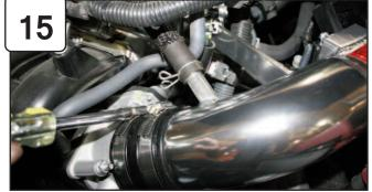
Tighten all clamps using 5/16" nut driver. Connect crank case line to tube.
