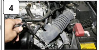
With 10mm socket or wrench loosen clamp on throttle body. Disconnect MAF sensor harness. Remove crank case line.
