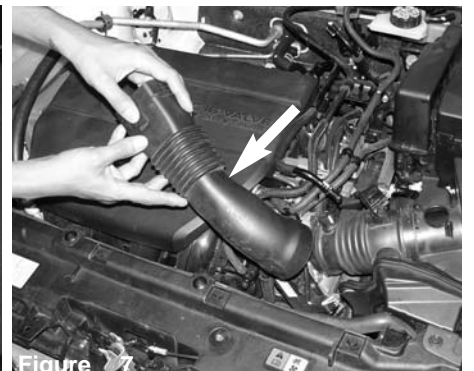
Figure 7 Carefully dislodge the plastic air intake duct from the air box cleaner and the throttle body.
