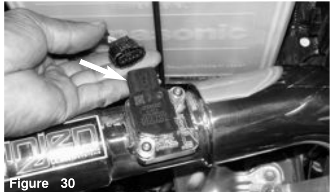
Figure 30 Press the electrical harness clip over the mass air flow sensor until it snaps in place.
