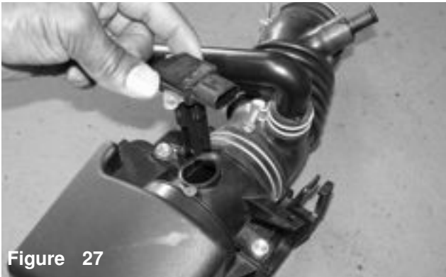
Figure 27 Once you have removed the two bolts, continue to pull the mass air flow sensor from the sensor housing.
