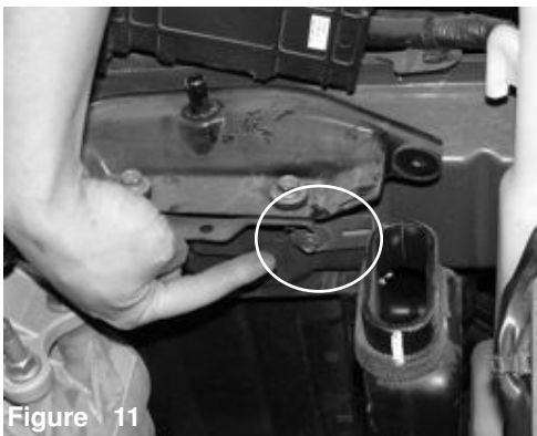
Figure 11 The m6 bolt is removed from the car frame. This bracket is attached to the plastic resonator box that will be removed. This is one of the three m6 bolts that will be removed.
