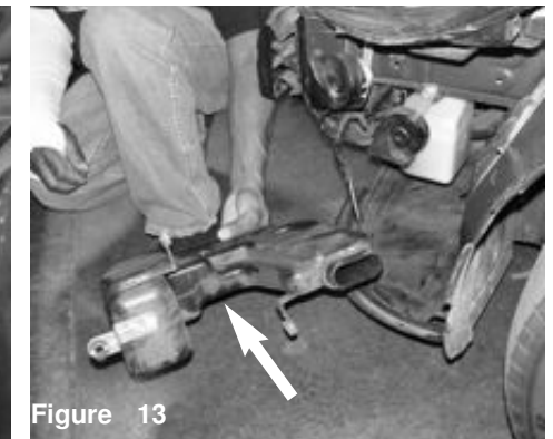
Figure 13 Once all three bolts have been removed, continue to pull the resonator box out.
