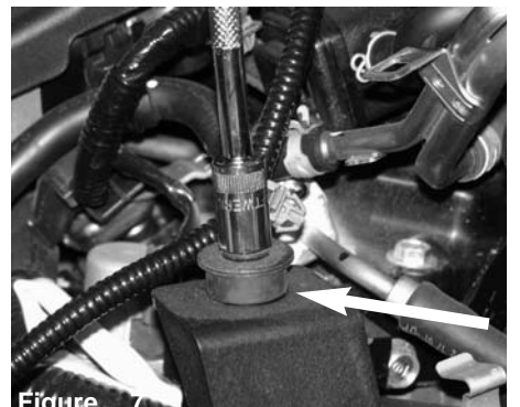
Figure 7 Loosen the screws holding the bottom half of air box using 10mm socket and ratchet.
