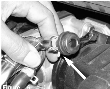
Figure 6 Carefully pull back the crank case linr away from air box.
