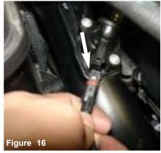
Disconnect the crank case line harness.
