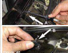
A) Loosen the bolt on left side of core support holding in headlight using T30 torx bit. B) Remove the bolt from vehicle.
