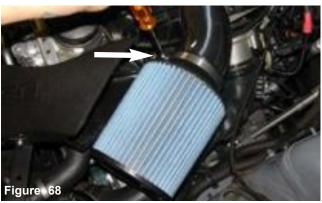
Install air filter to the tube and tighten and secure.
