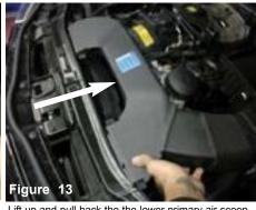
Lift up and pull back the lower primary air scoop assembly.
