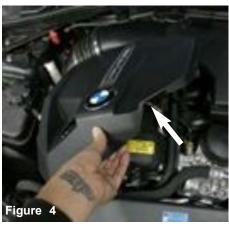
Carefully pull up and remove the engine cover.
