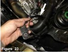
Remove the reservoir clamp from vehicle.
