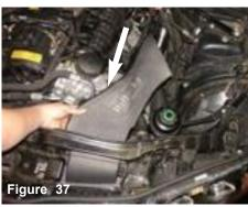
Install the driver side factory scoop, position the injen power-scoop to the back of the core support, locate the 2 inserts though the scoop. Secure the power-scoop using the 2 remaining M6 button head screws.
