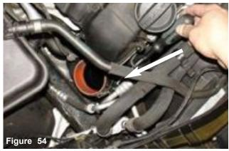
Secure the clamp on the turbo housing only using 8mm nut driver.
