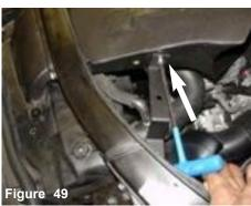
Install the Air scoop bracket to the power-scoop. secure using M6 button head screw.
