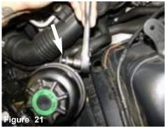
With 10mm ratchet and extension, loosen the screw holding in the reservoir clamp.
