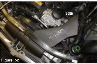
335i power-scoop and resovoir/air scoop bracket shown above. **Note:** Remaining steps will be the same for both the 135i and 335i.
