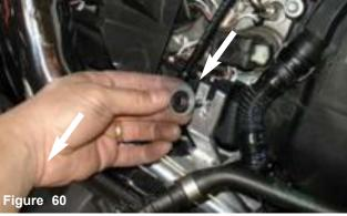
From step 15, use the factory bolt and provided fender washer to secure the bracket on engine. *Note: Make sure you use the fender washer.*
