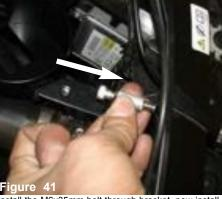
Install the M6x35mm bolt through bracket, now install the spacer to the bolt. Position the bolt to the back side of the thredded insert from previous step.
