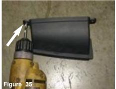
Drill all the 4 holes out to 1/4" on the factory scoops to make the M6 screws able to pass through.
