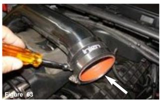
Install the  $3^\circ$  straight hose with clamps provided and attach to the end of the intake tube. Tighten on the tube only.
