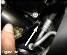
With T30 torx bit, loosen the screw holding in intake tube @ turbo housing.
