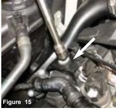
With 10mm socket and ratchet, loosen the bolt holding in the intake tube on engine and remove.
