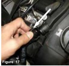
Carefully pull back the crank case fitting from the engine using a small flat head screwdriver.
