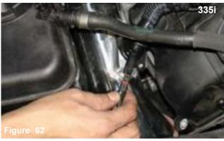
Connect the Crank case line harness.
