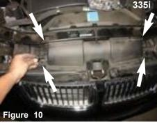
For the **335i** loosen and remove the 2 bolts and 2 plastic push clips holding in the primary 1 piece air scoop using t25 torx bit.
