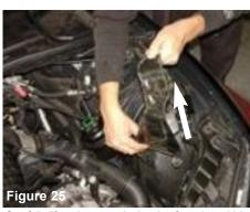
Carefully lift and remove the bracket from the vehicle.
