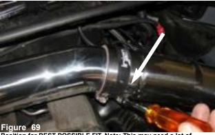
Position for BEST POSSIBLE FIT. Note: This may need a lot of adjustment with both tubes. Make sure that the hood has clearance and the tube is not touching the fuel line below.
