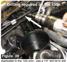
Applicable to the 135i only: Use a 1/4" drill bit to dril a hole through the composite cross member, the short bracket on the cup is used as a pattern.
