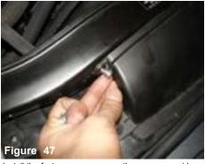
Install the factory scoop, secure the passenger side using the M6 button head screw and flange nut behind the core support.
