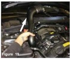
Carefully lift intake tube and slide back towards firewall and remove. *Make sure you remove the rubber gasket on turbo housing.*
