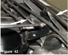
Make sure the spacer is used to preventing the bracket to distort. Tighten using allen key till bottoms out.
