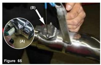
A) Install the MAF sensor into the new intake tube. B) Secure the MAF sensor using the provided M4 button head screws.
