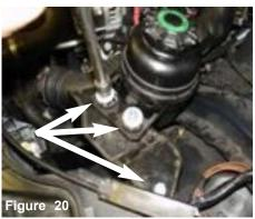
Loosen the 2 nuts holding in the power steering reservoir. Also, loosen the 10mm screw holding in the bracket.
