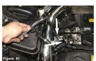
Secure the bracket and slide the slot on bracket forward so it stops and tighten using 10mm socket and ratchet.
