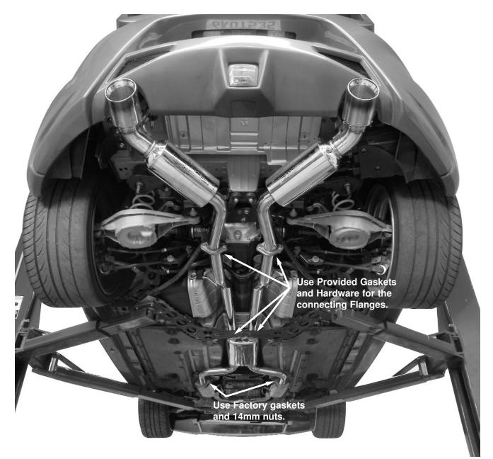
Step 1: Remove the factory Exhaust system using 14mm wrench or sockets. Save the 2 factory Gaskets at the Cats for re-use.
