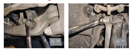
Make sure the lower fork/shock mount is fully seated against the shock adapter, install the nut and bolt and torque to 40Nm + 180 degree turn (29.5lb-ft + 180 degree turn) (fig. 36).
