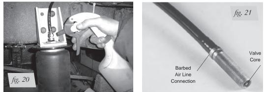
3. After the test, deflate the springs to the minimum pressure required to restore the Normal Ride Height, but not less than 10 PSI 4. IMPORTANT: Check the air pressure again after 24 hours. A 2 to 4 PSI loss after initial installation is normal. Retest for leaks if the loss is more than 5 lbs.
