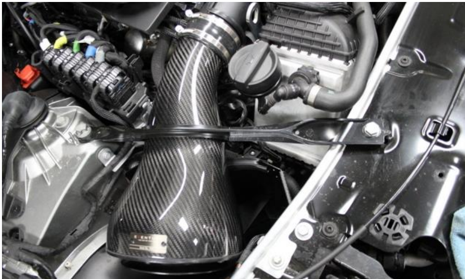
34. Now secure the strut brace with the 2 bolts. Repeat procedure for the LHS housing – you don't need the rubber strip from step 26 for the LHS housing.
