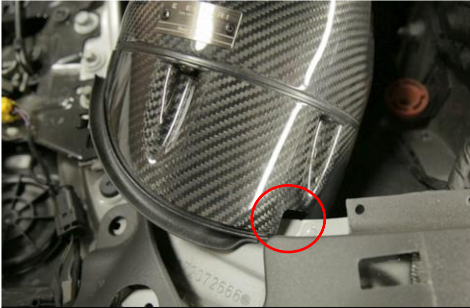
28b. Use the cut out in the shroud to gain more clearance as the housing is positioned into place,
