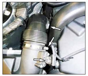
5. Disconnect the maf sensor electrical connection. Loosen the hose clamp that secures the factory intake tube to the air filter housing and then remove the air filter housing from the vehicle. Loosen the hose clamp that secures the factory intake tube to the turbo inlet pipe and then remove the tube from the vehicle. Stuff a towel into the turbo inlet pipe to prevent debris from falling into the turbo.
