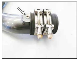
10. Install the provided 1/8npt accessory port plugs into the AEM charge tubes. NOTE: be sure to apply pipe sealant on the threads of the plugs. Install the provided couplers and clamps onto the charge tubes. NOTE: Slide the couplers all the way onto the pipes as shown as this will aid the installation of the pipes.
