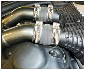
12. Slide the couplers onto the intercooler inlets, position the hose clamps and then tighten.
