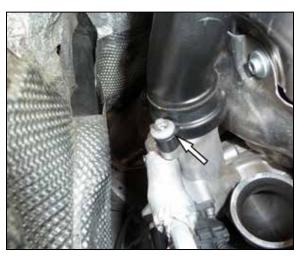
8. Remove the bolts that secure the factory charge tubes to the turbo and then remove the charge tubes from the vehicle. NOTE: The following size wrenches can be used to remove the TORX bolts, T50 TORX, 5/16" 12-point wrench, 8mm 12-point wrench.
