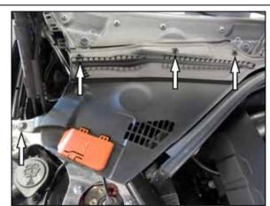
2. Remove the retaining pin and turn the three fasteners ¼ turn counterclockwise to unlock, then remove the cover panels from the vehicle.
