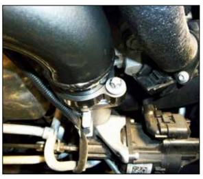
11. Install the AEM charge pipes onto the turbo and secure with the factory hardware from step #8.
