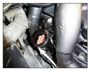
13. Reinstall the turbo inlet and secure with the factory hardware.
