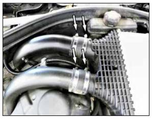
7. Loosen the four hose clamps the secure the factory charge tube hoses to the intercooler.
