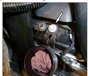
6. Remove the bolt that secures the turbo inlet pipe and then disconnect the pipe from the turbo and remove it from the vehicle.
