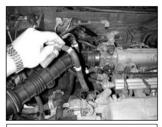
c. Detach the PCV hose from the fitting on the valve cover. Remove the hose assembly from the car.
