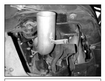
f. Line up the intake pipe support tab with the rubber mount. Install the rubber mount assembly as shown in the diagram below.
