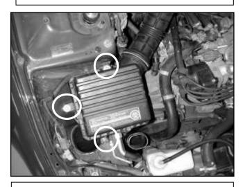
f. Remove the three air box mounting bolts and remove the factory air intake system from the car.
