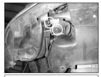
h. From underneath the car, remove the splash guard fasteners shown in the picture.
