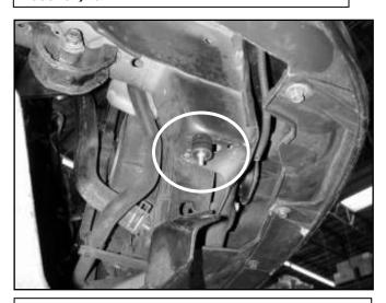
d. Thread the rubber mount into the hole on the bottom of the vehicle. (Hole that is exposed from the intake resonator removal during step 2j).
