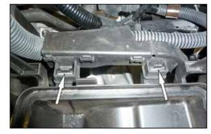
6. Release the two clips that secure the wiring harness to the lower air filter housing and then unhook the harness from the housing.
