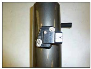
14. Remove the mass air sensor from the factory air filter housing and install it into the AEM® intake tube and secure with the provided hardware.
