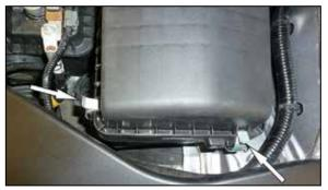
5. Release the two air filter upper housing clips and remove the upper housing, intake tube and air filter from the vehicle.
