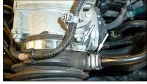
4. Release the spring clamp and disconnect the crank case vent line from the factory intake tube. Loosen the hose clamp that secures the factory intake tube to the throttle body.
