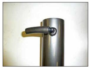
13. Install the 90° vent fitting and provided CCV hose into the AEM® intake tube as shown.
