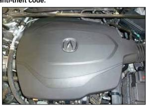
2. Lift the engine cover and remove it from the engine.
