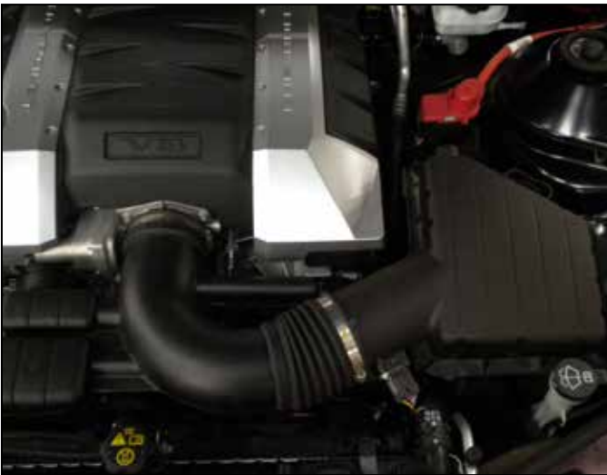
Factory air box system installed
