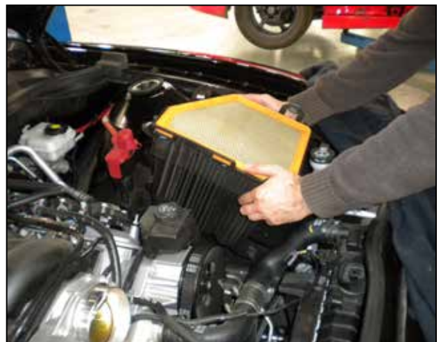
j. Carefully pull up on the lower box until it pops free from its retaining anchor. Make sure the rubber anchor stays in the frame rail as you will need it to install the AEM® intake system. Store the factory air intake system components and filter.
