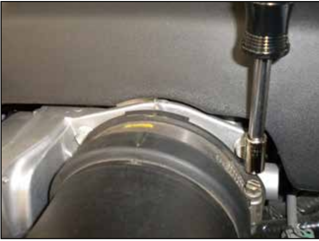
e. Loosen the large hose clamp at the engine throttle body.
