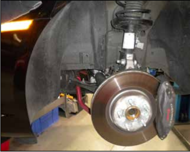
b. Remove the driver's side front wheel.
