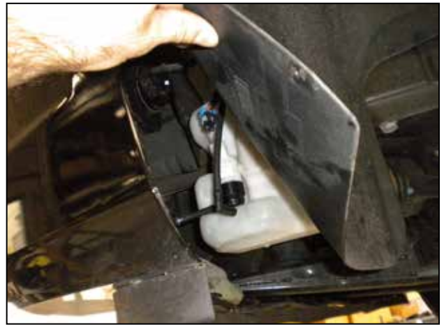
e. Carefully pull the fender cover away from the fender lip to gain access to the factory washer reservoir.
