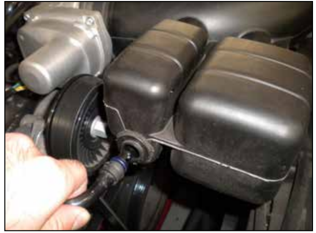
f. Disconnect the plastic breather pipe from the side of the factory intake resonator.
