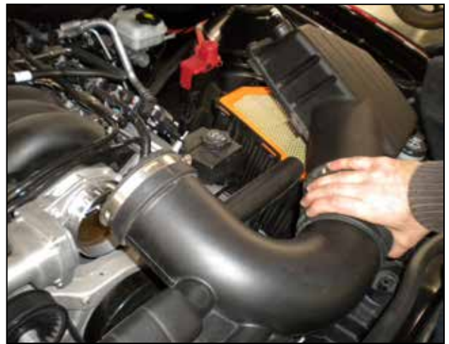
h. Remove the upper intake tube and air box lid from the engine bay. Remember, you will need the factory MAF sensor for the AEM® intake system.
