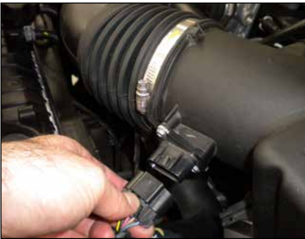
g. Disconnect the MAF sensor wire harness by depressing the tab and pulling the connector off.
