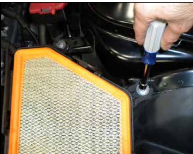
i. Remove the factory lower air housing; start by removing the two retaining nuts at the shock tower brackets. Retain the nuts for future use in a later step.
