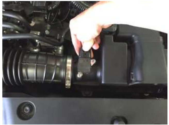
b. Disconnect the wiring harness to the mass airflow (MAF) sensor.
