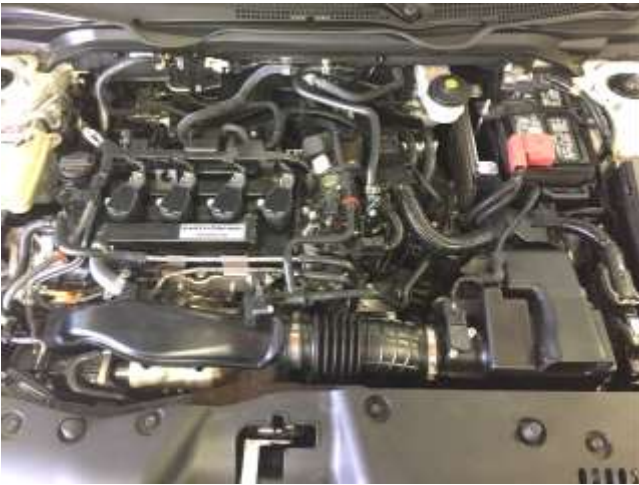
STOCK INTAKE INSTALLED
