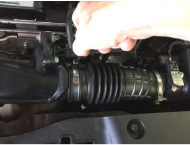
a. Using a small Phillips screwdriver or a 5.5mm socket, loosen the hose clamp retaining the original equipment (OE) inlet coupler and disconnect it from the turbo inlet.
