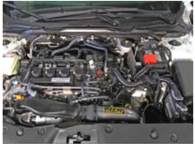
AEM INTAKE INSTALLED
