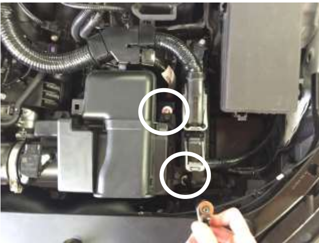
c. Use a 10mm socket with extension to fully loosen the bolts shown above which secure the factory air box. The air box may now be lifted out of the vehicle.
