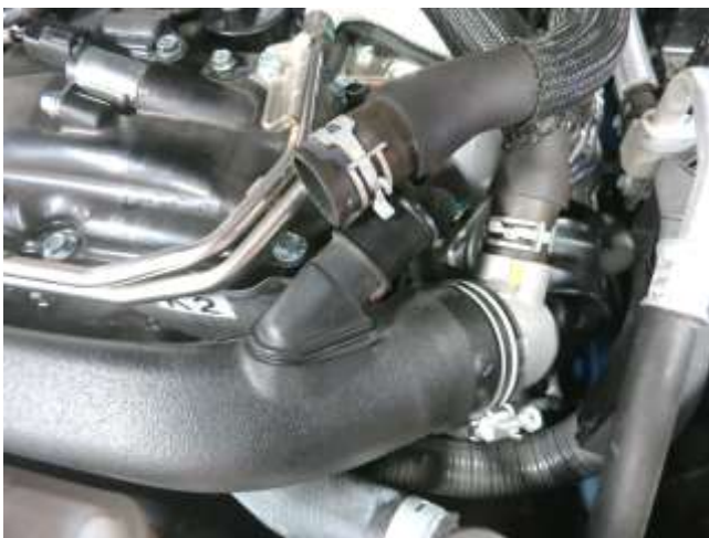
c. Use pliers to relieve tension on the hose clamp and then pull the breather hose off of the stock intake tube port.
