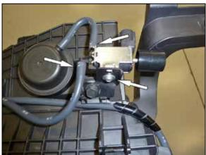
12. Remove the vacuum switching valve from the
