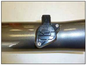
16. Remove the mass air sensor from the factory air filter housing and install it into the AEM® intake tube.
