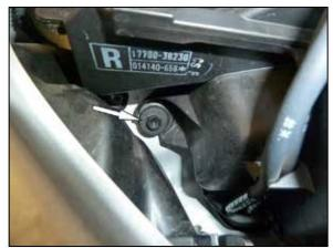
5. Remove the lower air filter housing mounting bolt.
