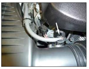
3. Disconnect the mass air sensor electrical connection and unhook the wiring harness.
