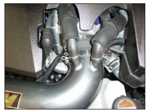
17. Install the AEM® intake tube through the heat shield and into the coupler on the throttle body. Adjust the tube for best fit and then secure with the
