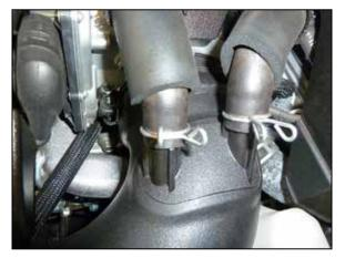
2. Release the spring clamps that secure the crank case vent lines and then unhook the vent lines from the factory intake tube. Loosen the hose clamp that secures the intake tube to the throttle body.
