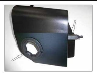
9. Install the 13.5" section of edge trim into the hole of the heat shield. Install the heat shield mounting post onto the heat shield using the provided hardware.
