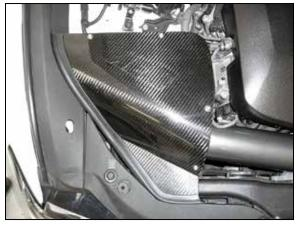
22. Install the carbon fiber lid assembly onto the heat shield and secure with the provided hardware.
