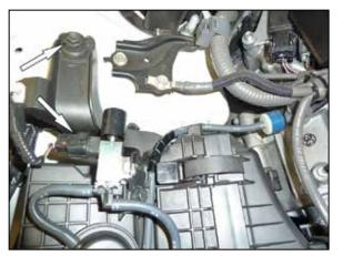
4. Disconnect the vacuum switching valve electrical connection. Remove the bolt which secures the air filter housing to the strut tower.
