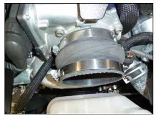
15. Install the provided hump coupler onto the throttle body and secure with the provided hose clamp.
