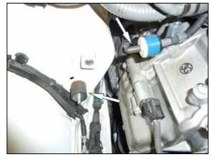
10. Install the provided vacuum cap onto the vacuum diaphragm. Install the provided rubber mounted stud into the strut tower as shown.
