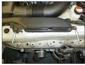
7. Remove the bolt and push pin that secure fresh air intake duct, then remove the fresh air duct and air filter housing from the vehicle.
