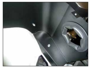
11. Set the heat shield into position in the vehicle so that the mounting stud inserts into the factory mounting grommet. Secure the heat shield to the rubber mounted stud with the provided hardware.
