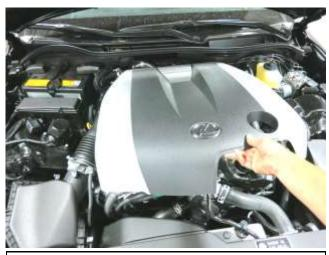
a. Lift up on the engine cover to loosen and carefully set it aside.
