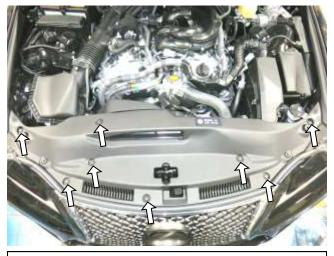
b. Depress the 8 plastic clips indicated and remove the plastic upper fascia.
