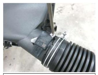
h. Use a Philips screwdriver to remove the MAF sensor from the stock intake tube.
