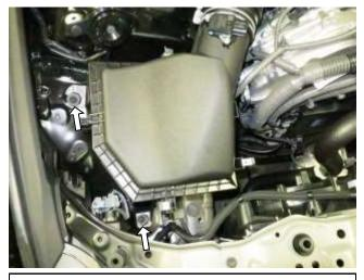
f. Loosen and remove the two M6 bolts indicated.
