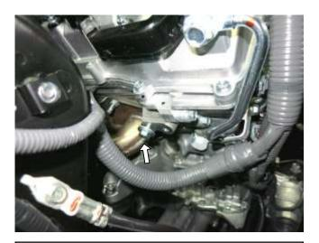
c. Loosely install the provided M8 bolt(1-2066) and washer(559960) into the threaded hole located on the engine block.
