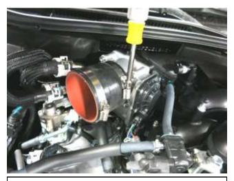
f. Install the provided coupler (5-323 for IS250 models and 5-325 for IS350 models) and fasten the hose clamp over the throttle.
