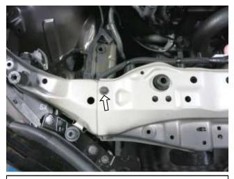
b. Remove the indicated bolt using a 10mm socket. Set this bolt aside for use with the AEM heat shield installation.
