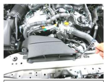
c. Use a 10mm socket to remove the M6 bolt securing the fresh air inlet duct. Detach the air duct from the lower airbox and set aside.
