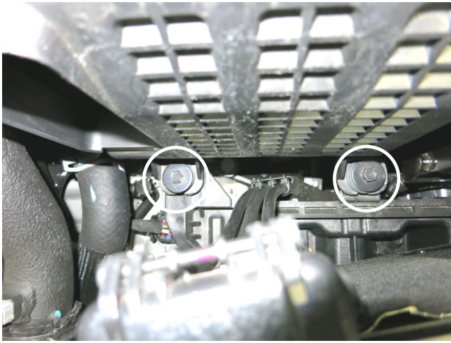
f. Remove the two bolts securing the air box to the vehicle. These will not be reused.
