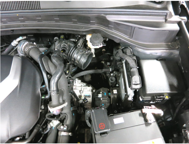
g. Remove the stock air box from the vehicle. Note: Do not discard any of your stock equipment.
