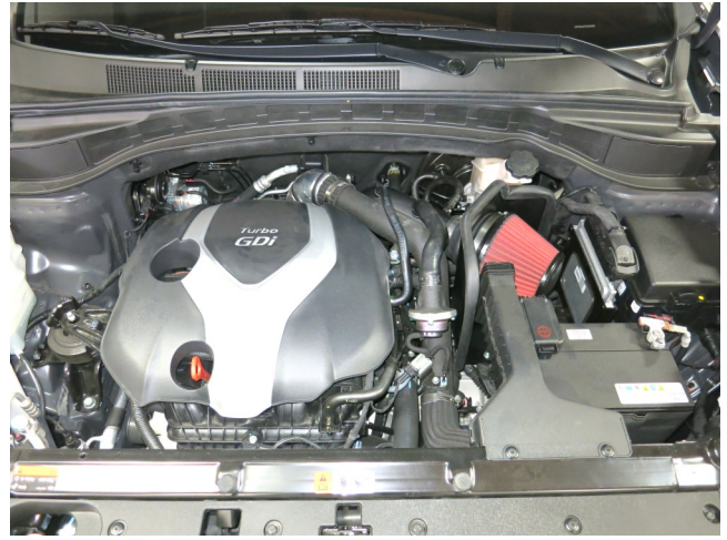
AEM INTAKE INSTALLED
