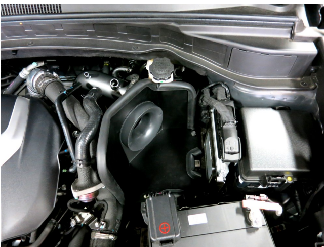
g. Install the assembled heat shield into the vehicle aligning the two slots with the previously installed rubber mounts. Push down to secure the stand-off.
