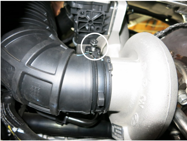
h. Loosen the hose clamp securing the stock intake tube to the turbo compressor housing.
