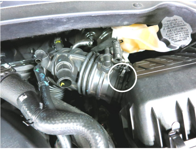
e. Loosen the bolt hose clamp securing the stock intake tube to the air box.
