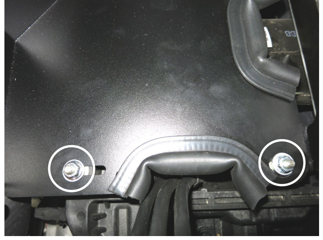
h. Install the washers and nuts, then tighten them to the rubber mounts.
