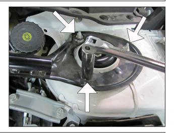
d. Remove the strut mount brace by removing the three 14mm nuts at each strut tower. Once all the retaining nuts have been removed, remove the strut brace from the engine bay and set it aside.
