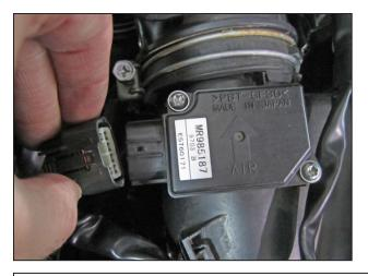
k. Disconnect the wiring harness connector from the MAF sensor.
