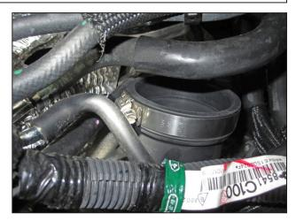
k. Install the elbow coupler (5-1057) to the turbocharger compressor inlet as shown. Tighten the smaller
