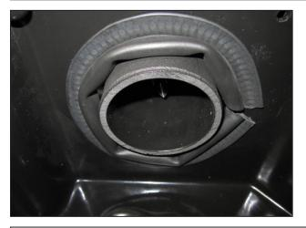
n. Align the intake tube by centering it inside the large air box outlet hole as shown. Once it is aligned, carefully remove the air box.
