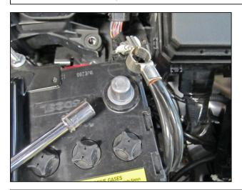
c. Disconnect the negative battery cable.
