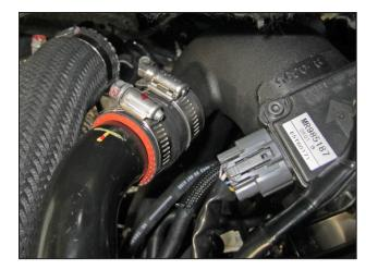
ad. Connect the turbo wastegate bypass pipe to the silicone hose (5-1055) as shown and secure in place with a #28 hose clamp (103-BLO-2820).
