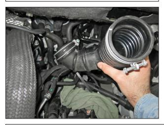
u. Unfasten the lower hose clamp at the turbo inlet and remove the lower intake tube from the turbocharger.
