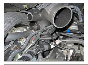
I. Install the upper intake tube onto the large end of the elbow coupler as shown. Tighten the upper #48 hose clamp, but not completely so the intake tube can rotate slightly.
