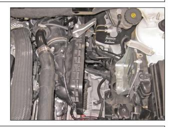
h. Remove the right half of the air box assembly by sliding it up and off of the two mounting studs.
