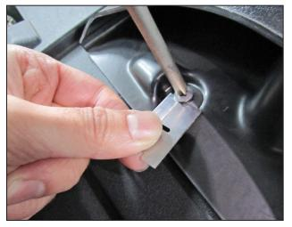
a. Remove the threaded retaining clips at the intake scoop inlet using a Philips screwdriver. You may need to pull the scoop to one side to provide a side load, or push on the side of the plastic screw as shown, forcing the screw threads to "catch" and climb out of the insert. Remove the intake scoop.
