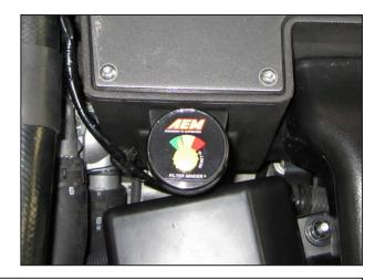
ak. Ensure the needle on the AEM<sup>®</sup> filter minder gauge is set to the "Green" section on the indicator.
