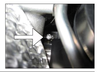
o. Completely tighten the lower #36 hose clamp securing the elbow coupler to the turbo inlet. Ensure the elbow coupler is fully seated on the turbo inlet.
