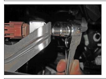
m. Remove the 10mm nut that holds the turbocharger wastegate solenoid to its metal bracket on the air box. The nut will be reused during the installation of the AEM<sup>®</sup> intake system.
