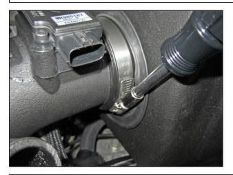
x. Slide the #52 hose clamp over the flange of the filter on the outside of the air box. Tighten the hose clamp on the outside of the air box as shown.
