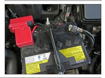
ag. Reconnect the negative battery cable to the battery.
