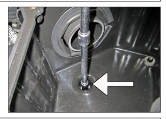
u. Re-install the AEM<sup>®</sup> air box, following the installation procedure specified in Step 3m. Ensure the air box is properly mounted and aligned and secure to the shift cable bracket. Ensure the AEM<sup>®</sup> intake tube's inlet is centered in the air box outlet.
