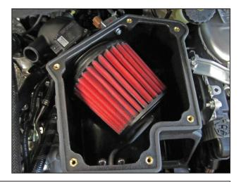
w. Install the AEM<sup>®</sup> air filter by pushing it through the edge trim and onto the intake tube's inlet. Ensure the air filter is properly seated onto the intake tube.
