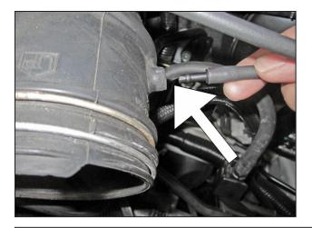
q. Locate the short black hose that runs from the turbo wastegate solenoid to the intake tube. Disconnect the short black hose from the turbo wastegate solenoid.
