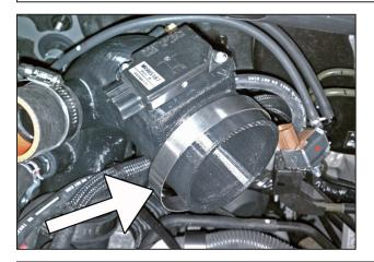
t. Place a #48 hose clamp (9452) onto the open inlet of the intake tube (9-0395) as shown.
