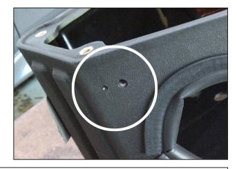
aa. Note the small alignment dimple next to the wastegate solenoid mounting hole on the AEM<sup>®</sup> air box. When the wastegate solenoid is mounted to the air box ensure the alignment tab (Pointed out in Step 3z) aligns in the dimple.
