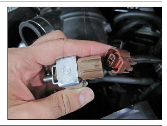
n. Disconnect the wastegate solenoid from its wiring harness. Disengage the long black solenoid hose from the 2 rubber retainers along the side of the intake tube, but leave connected to the solenoid. Set the solenoid aside in a safe area.
