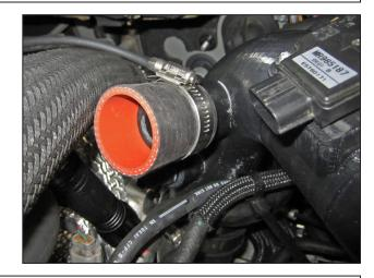
s. Install the silicone hose (5-1055) onto the AEM<sup>®</sup> intake tube. Attach the silicone hose about 1/3 of the way onto the turbo bypass port. Secure in place with a #28 hose clamp (103-BLO-2820).
