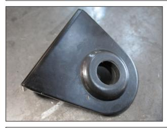
h. Install the rubber grommet (784634) in the filter minder bracket (32-3017) as shown.
