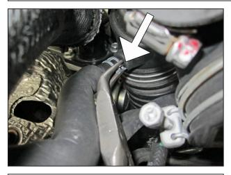
s. Disconnect the breather hose from the intake tube.
