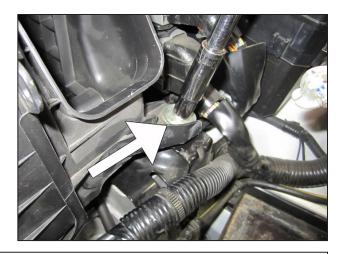
f. Remove the washer and mounting bolt retaining the front of the stock air box.
