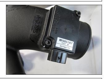
e. Mount the stock MAF sensor onto the upper intake tube (9-0395) using the provided M4 Allen bolts. **NOTE: Ensure the MAF sensor is properly installed so the arrow indicating AIR FLOW is oriented as shown.**
