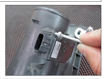
p. Remove the MAF sensor from the air box outlet tube. The MAF sensor will be reused in a later step during the installation of the AEM<sup>®</sup> intake system.
