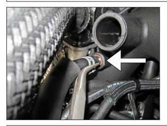
r. Install the valve cover breather hose onto the ¼" barbed vent installed on the AEM<sup>®</sup> intake tube. Secure the valve cover breather hose with the stock hose clamp.
