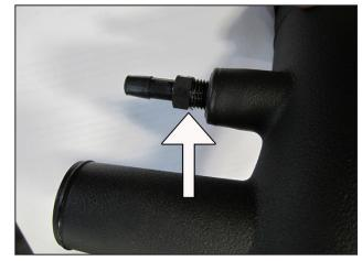
c. Install the 3/8" NPT barbed vent (08047) into the upper intake tube's (9-0395) boss and fully tighten."
