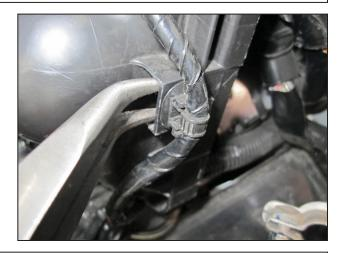
j. Unfasten the 3 plastic clips retaining the MAF wiring harness to the left half of the air box with a pair of pliers.
