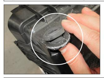
i. Remove the 2 rubber isolator grommets from the bottom of the right half of the air box assembly. These will be reused during the installation of the AEM<sup>®</sup> intake system.
