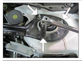
af. Install the strut brace, securing the 6 mounting nuts to their factory torque specification (33 +/- 5 lb-ft).
