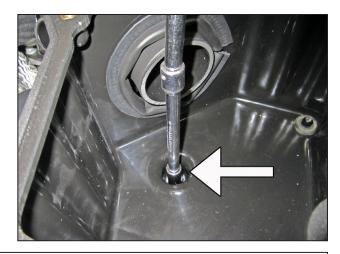
m. Install the AEM<sup>®</sup> air box, ensuring the 2 isolator grommets are mounted and fully seated on the mounting studs. Using the stock bolt removed in step 2v and a washer (1-3022), align the air box and secure to the shift cable bracket. Ensure the AEM<sup>®</sup> intake tube's inlet is centered in the air box outlet. Do not fully tighten!
