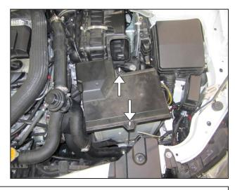
b. The vehicle's battery is located under the stock intake scoop. Remove the plastic retaining nuts and battery cover to access the battery.
