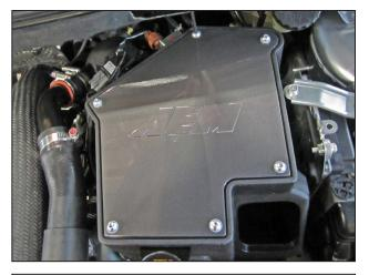
ae. Install the aluminum heat shield lid onto the air box top. Secure the heat shield lid in place using the 6 plastic washers (1-3001) and 6 buttonhead bolts (1-112). Install all the hardware before completely tightening. Once the heat shield lid is properly aligned, fully tightening the hardware by starting at the back of the air box and moving in a clockwise direction.
