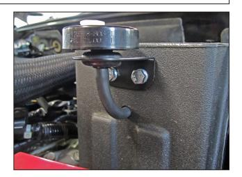
y. Locate the hose (5-3009) attached to the AEM<sup>®</sup> air filter and route the hose through the hole in the air box below the AEM<sup>®</sup> filter minder gauge. Connect the hose to the gauge's outlet. Trim any excess hose.
