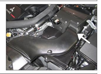
ai. Install the stock intake scoop into the matching inlet of the  $\text{AEM}^{\circledast}$  air box and over the battery cover.
