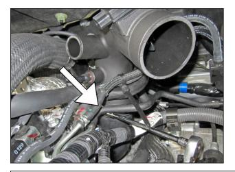
p. Completey tighten the #48 hose clamp securing the upper intake tube to the elbow coupler. Ensure the upper intake tube is fully seated into the elbow coupler.
