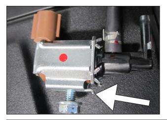
z. Make note of the small alignment tab at the base of the wastegate solenoid.
