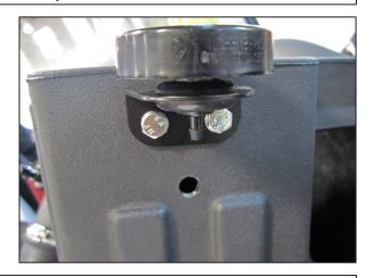
i. Insert the filter minder gauge onto the filter minder bracket (32-3017). Attach the filter gauge assembly onto the air box using the two M6 hex bolts (1-2065) and two split washers (1-3025) as shown.
