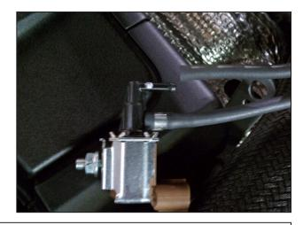
r. Completely remove the small black hose from the upper solenoid port.
