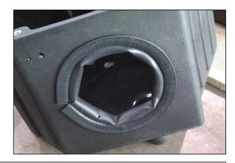
g. Install the edge trim (8-4015) around the large outlet in the air box as shown. Trim the edge trim if necessary.
