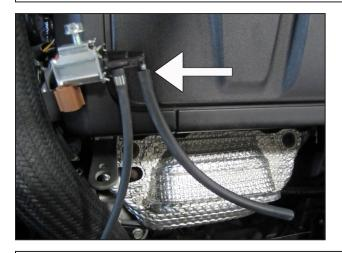
j. Install the supplied black hose onto the upper port of the wastegate solenoid as shown.
