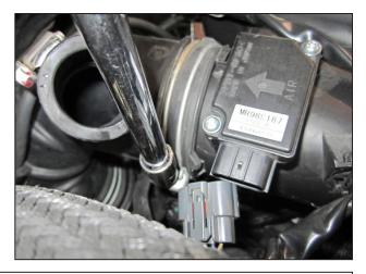
I. Locate the hose clamp securing the air box outlet to the intake tube and unfasten.
