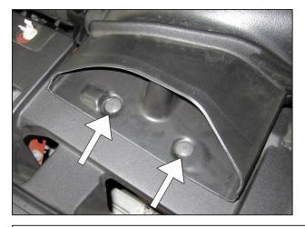
aj. Re-install the plastic retaining clips to secure the inlet of the intake scoop.
