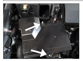
ah. Replace the battery cover and retaining nuts removed in step 2b.
