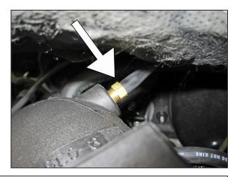
q. Install the loose end of the hose attached to the wastegate solenoid onto the smaller 1/8" barbed vent of the AEM® intake tube as shown. Trim the hose if necessary.
