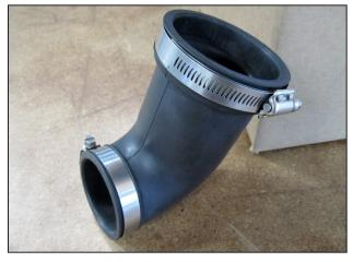
b. Place the #36 hose clamp (9436)over the small end of the flexible elbow coupler (5-1057). Slide the #48 hose clamp (103-BLO-4820) over the large end of the elbow coupler.
