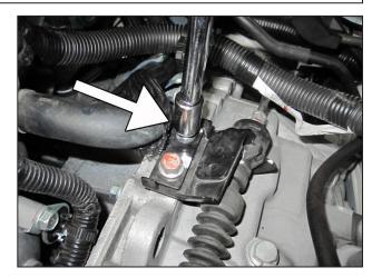
v. Locate the shift cable bracket on top of the transaxle case. Remove the specified 12mm bolt securing the shift cable bracket. This bolt will be reused in a later step during the installation of the AEM<sup>®</sup> intake system.
