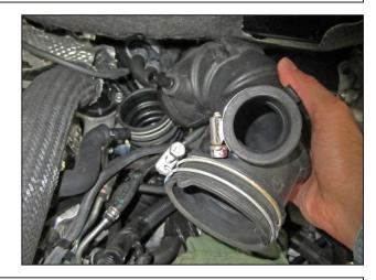
t. Unfasten the middle hose clamp and remove the upper intake tube from the lower tube.
