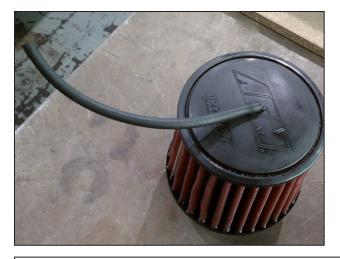
v. Install the provided elbow fitting (8-152) into the AEM<sup>®</sup> air filter's top (21-2031D-H). Install the provided hose (5-3009) onto the end of the elbow port as shown.
