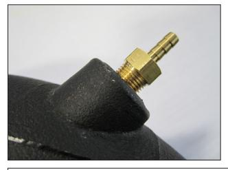
d. Install the smaller NPT barbed vent (087016) into the upper intake tube's other boss and fully tighten.
