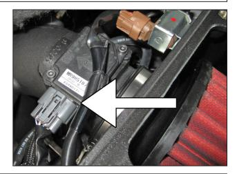
ac. Connect the stock wiring harness to the MAF sensor and the stock wiring harness to the wastegate solenoid.
