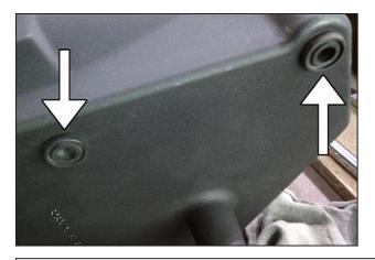
f. Install the 2 rubber isolator grommets removed from the stock air box into the two large holes on the base of the AEM<sup>®</sup> air box (9-0393).
