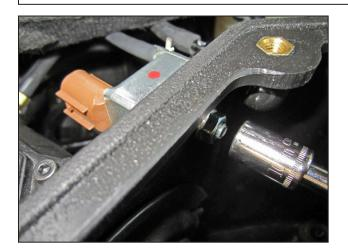
ab. Mount the wastegate solenoid to the hole on the back side of the AEM<sup>®</sup> air box using the stock 10mm nut. Align the solenoid's small tab with the dimple next to the mounting hole and fully tighten the nut to secure the solenoid to the air box.
