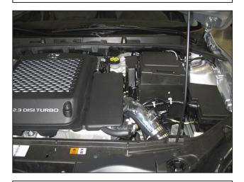
AEM® intake system installed
