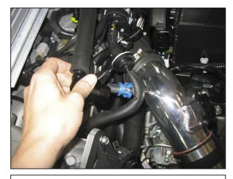
f. Install the upper intake pipe into the 45-degree coupler on the turbo inlet. Rotate the intake pipe until the breather hose aligns with the intake pipe's nipple. Attach the breather hose to the intake pipe nipple and connect the MAF sensor harness connector to the MAF sensor.
