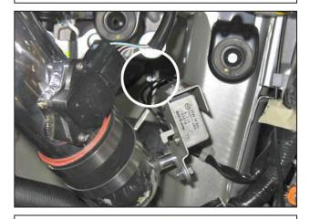
k. Secure the lower intake pipe's mounting bracket to the rubber mount with a M6 washer and nut. Reconnect the wiring harness to the resistor ballast.
