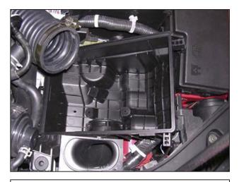
f. Remove the check tab on the backside of the air filter housing, then slide the rubber isolator rearward. Lift up on the lower air filter housing and remove.
