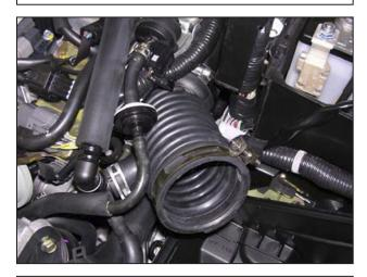
g. Disconnect the plastic breather hose from the inlet tube by squeezing the blue retaining clip and pulling on the breather hose. Loosen the hose clamp on the turbo inlet and remove the tube.
