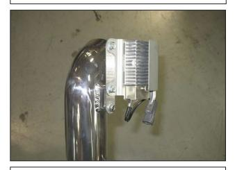
i. Attach the resistor ballast to the lower intake pipe using the mounting bracket, three M6 bolts, three washers, and one M6 nut.
