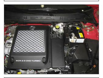
Factory air box system installed
