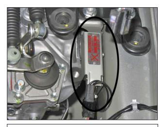
g. Locate the resistor ballast for the headlight on the inside of the driver's side frame rail. Unplug the wiring harness and remove the two bolts securing it in place.
