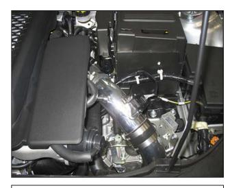
m. Reinstall the intercooler cover and check for clearance. Adjust the intake pipes if necessary.
