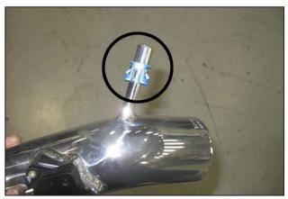
c. Install the plastic breather hose clip (removed in step 2I) onto the nipple of the upper intake pipe. Simply slide the clip over the end until it snaps into place.
