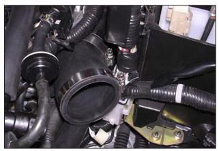
b. Install the 45-degree coupler onto the turbo inlet and secure using a #40 hose clamp.
