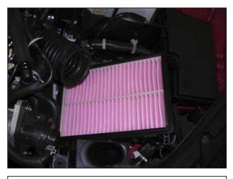
d. Unclip the two metal retaining straps securing the air filter housing lid to the lower air box housing. Loosen the hose clamp securing the inlet tube to the turbo inlet pipe and remove the lid.
