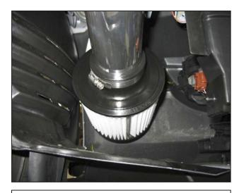
I. Install the air filter onto the end of the lower intake pipe. Push the air filter over the intake pipe until the stop in the air filter is reached. Secure the air filter onto the intake pipe with a #48 hose clamp.
