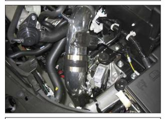
j. Install the lower intake pipe into the coupler of the upper intake pipe, and secure in place with a #44 hose clamp. Align the intake mounting bracket with the rubber mount that was installed in the step 3h.
