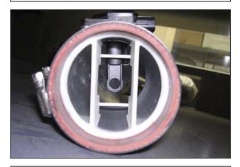
e. Slide the airflow straightener through the coupler and into intake pipe, aligning the slots with the MAF sensor as shown.
