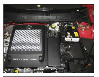
b. Remove the two bolts securing the plastic intercooler shroud. Remove the shroud.
