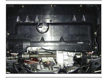
h. From underneath the vehicle remove the seven bolts and two plastic connectors securing the center splash shield in place, then remove the center splash shield.
