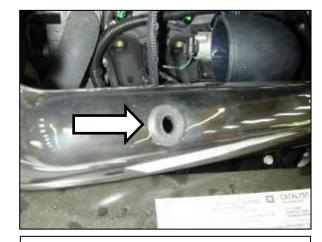
i. Insert supplied grommet into inlet pipe.
