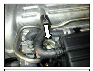
d. Release the spring clamp on the breather hose and pull hose off of the valve cover.
