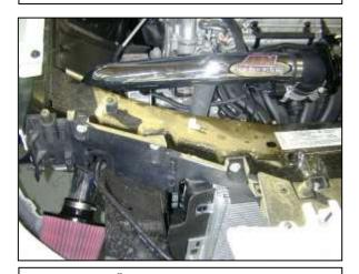
AEM® intake system installed
