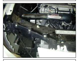
j. Install the intake pipe in engine bay as shown. Route the pipe up through the fender well into the engine bay.
