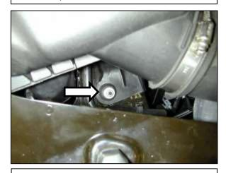
f. Remove the nut located behind headlight.
