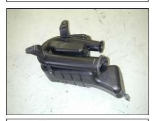
m. Remove the lower air box from the vehicle.
