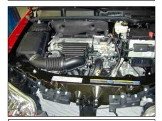
Factory air box system installed.
