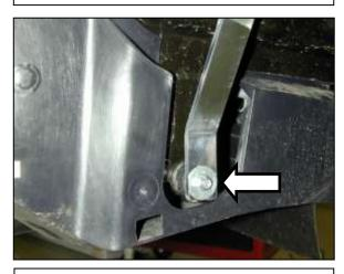
I. Place the lower support tab under the fender washer.
