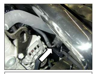
o. Insert IAT sensor through the grommet in the inlet pipe. Be careful not to push the grommet into the pipe.
