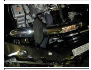
q. If an AEM® bypass valve is installed, install the bypass valve as shown. The intake pipe will require some modification to accommodate the AEM bypass valve. Follow the instructions included with the bypass valve for proper installation.
