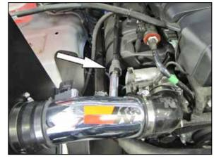
20. Connect the crank case vent hose to the fitting installed into the K&N $^{\!0}$  intake tube.
