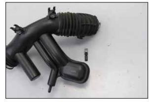
27. Remove the inlet air temperature sensor from the factory intake plenum as shown. NOTE: Use caution working with the inlet air temperature sensor as it is very fragile.
