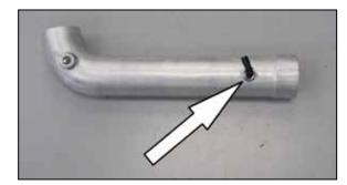
25. Install the 90°,  $\frac{1}{2}$ " vent fitting into the K&N<sup>®</sup> intake tube as shown.
