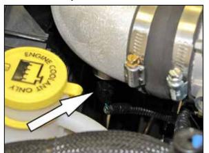
33. Reconnect the inlet air temperature sensor electrical connection and then reinstall the engine
