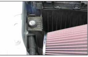
20. Install the rubber mounted stud into the into the air box mounting plate bolt location as shown.
