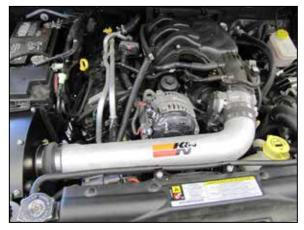
31. Install the K&N<sup>®</sup> intake tube into the silicone hose at the filter adapter and then into the hose at the throttle body, then secure with the provided hose clamps.
