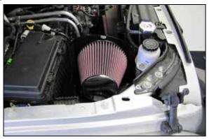
17. Install the K&N $^{\circ}$  air filter onto the filter adapter and secure with the provided hose clamp.
