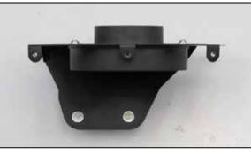
13. Install the provided filter adapter onto the heat shield as shown.
