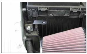
21. Install the provided bracket (083163) onto the rubber mounted stud using the provided hardware.
