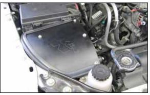
22. Install the K&N<sup>®</sup> filter lid and secure with the provided hardware.
