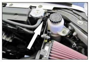
19. Install the heat shield bracket assembly onto the heat shield and radiator mount as shown. Secure the bracket with the factory bolt from step number 9 and the hardware provided.
