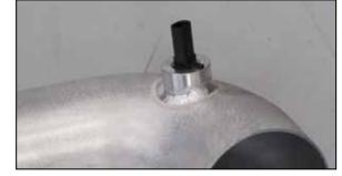
28. Install the inlet air temperature sensor into the  $K\&N^{\otimes}$  intake tube as shown.
