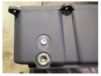
Locate the threaded boss inside of the transmission pan. Set the 2" magnet over the boss and secure it in place using the supplied M 6x10mm bolt and M6 lock washer.
