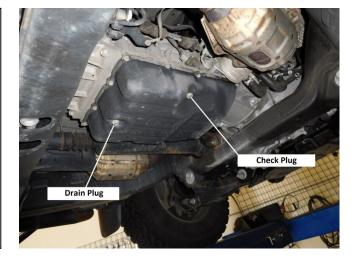
2. When installing new drain plug we recommend using sealant tape on the threads.
