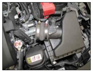
4. Install the provided hump coupler (08171) onto the filter housing and secure with the provided hose clamp. 5. Install the provided coupler (08690) onto the throttle body and secure with the provided hose clamp.
