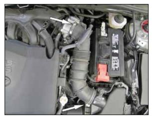
2. Loosen the hose clamps that secure the factory intake tube to the throttle body and air filter housing. Disconnect the two vent lines that connect to the intake tube and then remove the factory intake tube from the vehicle.
