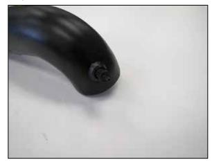
6. Install the provided vent fitting into the K&N $^{\mbox{\scriptsize \$}}$  intake tube as shown.
