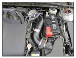
7. Install the K&N<sup>®</sup> intake tube into the coupler at the throttle body and then into the coupler at the air filter housing, adjust the tube for best fit and then secure with the provided hose clamps. Connect the crank case vent line to the fitting installed into the K&N<sup>®</sup> intake tube.
