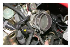
17. Install the provided silicone hose onto the throttle body and secure with the provided hose clamp.
