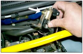
31. Remove the factory bracket from the purge control valve and replace it with the new K&N® "L" bracket using the stock nut.
