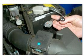
2. Disconnect the mass air sensor and air temperature sensor electrical connections.
