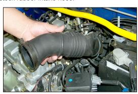
5. Loosen the hose clamps at the throttle body and at the mass air sensor, then, remove the rubber intake hose.
