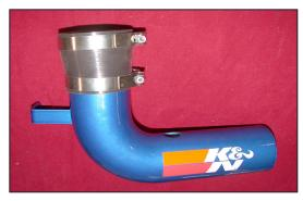
24. Install the remaining step hose and hose clamps onto the K&N<sup>®</sup> intake tube but do not tighten completely.
