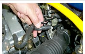
4. Disconnect the crank case vent hose from the stock rubber intake hose.
