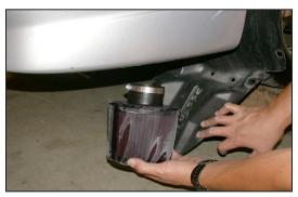
35. From underneath the vehicle install the K&N® air filter onto the K&N® cold air intake tube and secure with the provided hose clamp.
