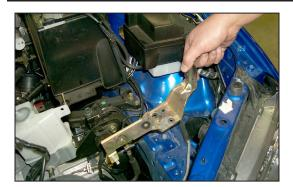
10. Loosen and remove the two bolts that secure the coolant reservoir support bracket to the inner fender, then, remove the support bracket.
