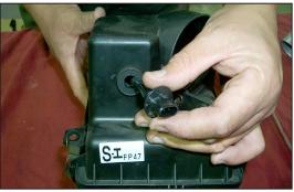
13. Remove the air temperature sensor from the air cleaner lid as shown.
