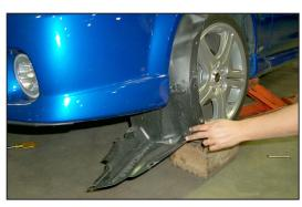
11. Jack the vehicle up and support it with jack stands, then, remove the inner fender wheel house valance as shown.
