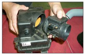
12. Loosen and remove the two bolts that secure the mass air sensor to the air cleaner lid, then, remove the mass air sensor.
