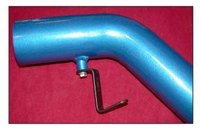
27. Install the "Z" bracket onto the threaded boss on the K&N® cold air intake tube and secure with the provided hardware.
