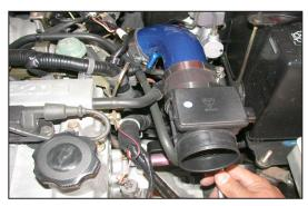
22. Slide the K&N® throttle body tube into the silicone hose on the throttle body, but do not tighten at this time.
