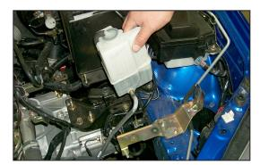
9. Slide the coolant reservoir upwards to release the reservoir from the support bracket as shown.
