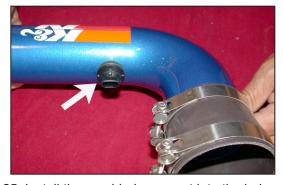
25. Install the provided grommet into the hole on the K&N $^{\otimes}$  "L" tube, then, install the air temperature sensor into the grommet.
