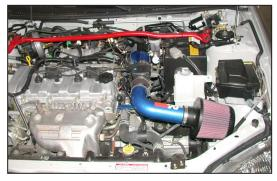
39. This K&N® high flow intake system has been designed to be used in two different configurations. In the case of inclement weather, the cold air tube can be removed and the air filter can be clamped onto the intake tube located in the engine compartment to avoid the possibility of ingesting water into the engine.
