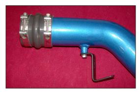
28. Install the silicone hump hose onto the cold air intake tube and secure with the provided hose clamp.
