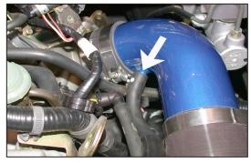
33. Reconnect the crank case vent hose to the K&N® intake tube as shown.
