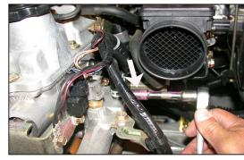
23. Secure the mass air bracket to the original fuel line support bracket using the bolt removed in step 20
