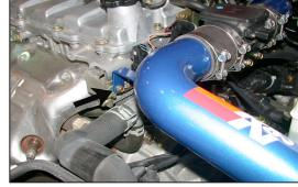
26. Slide the K&N® "L" tube onto the mass air sensor and line up the tube bracket with the ground bracket and secure with the stock bolt.
