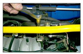
32. Secure the purge control valve to the bracket/ threaded boss on the intake manifold using the stock hex bolt.
