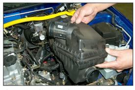
7. Loosen and remove the nut and bolt that secure the air cleaner assembly, then, remove the air cleaner assembly.
