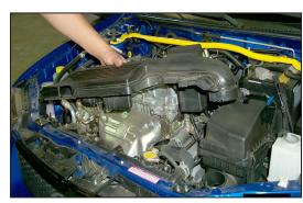
6. Loosen and remove the two nuts that secure the air inlet ducting to the top of the radiator core, then, remove the air inlet ducting.
