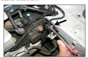
14. Remove the upper bolt on the transaxle mount as shown
