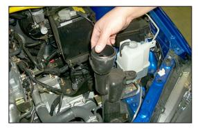
8. Loosen and remove the secondary air inlet duct that attaches to the air cleaner assembly and remove.
