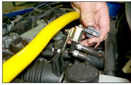
3. Remove the purge control valve from the stock rubber intake tube.
