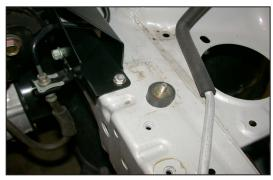
29. Install the rubber mounted stud into the threaded hole on the inner frame rail as shown.
