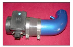
19. Slide the mass air sensor into the silicone step hose on the throttle body tube and secure with the provided hose clamp, but do not tighten completely. Note: Make sure the direction of the airflow is towards the throttle body as indicated by the arrow located on the mass air sensor.
