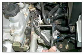
20. Remove the bolt that secures the fuel line support bracket as shown.
