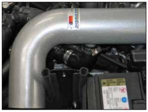
23. Feed the air injection hose assembly under the tube and mounting bracket and then connect the Open end of the air injection hose to the K&N® intake tube and secure with the provided hose clamp.
