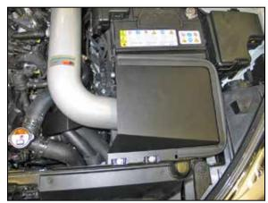
27. Install the cover onto the heat shield and then secure it to the heat shield and core support with the hardware provided.
