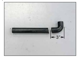
20. Cut the provided  $90^{\circ}$  air injection hose as shown. The hose should be  $3^{\circ}$  long.
