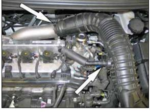
4. Release the spring clamp securing the crank case vent hose and then disconnect the crank case vent hose. Loosen the hose clamp securing the intake hose to the turbo inlet and then disconnect and remove the intake hose from the vehicle.
