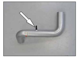
18. Install the provided Vent fitting into the  $K\&N^{\otimes}$  intake tube as shown.
