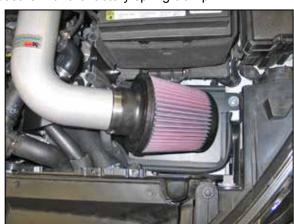
25. Install the K&N® air filter and secure with the
