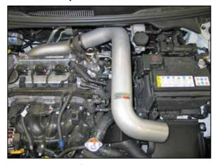
19. Install the K&N® intake tube into the silicone hose and align with the mounting bracket. Secure the tube with the hose clamp and hardware provided.
