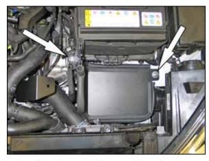
16. Install the heat shield assembly and secure it the two air box mounting locations with the provided hardware as shown.
