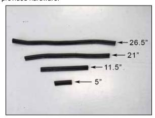
13. Cut the provided edge trim into four sections, One section will be 26.5" long, one section will be 21" long, one section will be 11.5" long and the final section will be 5" long.
