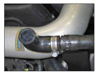
22. Connect the 90° air injection hose to the factory injection hose as shown and secure with the provided hose clamp.
