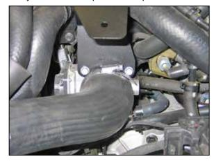
11. Reinstall the inlet charge hose onto the throttle body and secure with the factory hose clamp.
