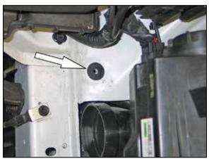
15. Set the provided rubber fender washer onto the air box mounting location on the inner fender as shown.
