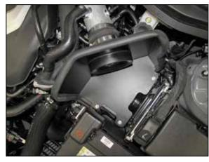
17. Set the heat shield into position on the rubber mounted studs and secure with the provided hardware.
