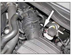
4. Loosen the hose clamp securing the intake hose to the air hox
