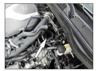
7. Install the provided 90° elbow hose (08504) onto the turbo inlet and secure with the provided hose clamp.
