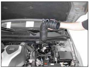
6. Loosen the hose clamp securing the intake tube to the turbo inlet and then remove the intake hose from the vehicle.
