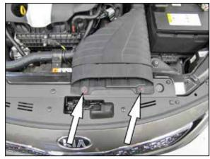
2. Remove the two bolts that secure the fresh air intake scoop to the core support and then remove the fresh air intake scoop from the vehicle.
