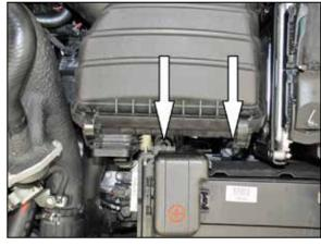
5. Remove the two bolts securing the air box to the mounting bracket. Then remove the air box from the vehicle.
