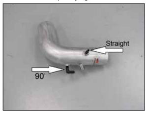
8. Install the provided  $90^{\circ}$  and straight vent fittings into the K&N® intake tube as shown.
