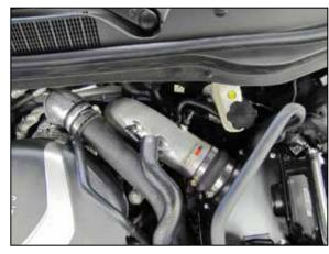
18. Align the intake tube with the filter adapter and slide the silicone hose onto the adapter. Tighten all of the hose clamps for the upper and lower silicone hoses securing the intake tube.
