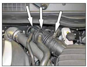
3. Loosen the spring clamps and then disconnect the Blow off valve hose, EVAP hose and Crank case vent hose from the intake tube.
