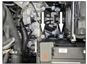
10. Install the two ½" high rubber mounted studs provided into the air box mount bolt locations.
