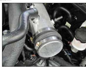
16. Slide the silicone hose (08699) onto the intake tube all the way on. Do not tighten at this time.
