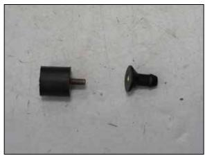
11. Install the provided 1" high rubber mounted stud into the heat shield mounting stud.
