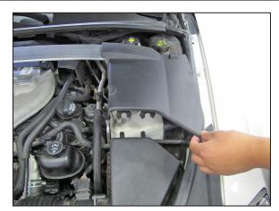
3. Lift up the front of the side cover and then remove the cover from the engine compartment.
