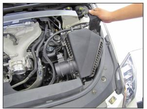
Remove the air filter housing from the vehicle.
