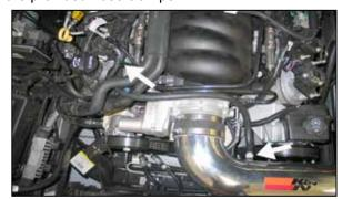
22. Attach the provided crank case vent hose to the 1/4npt fitting and then attach the open end to the vent port on the valve cover.
