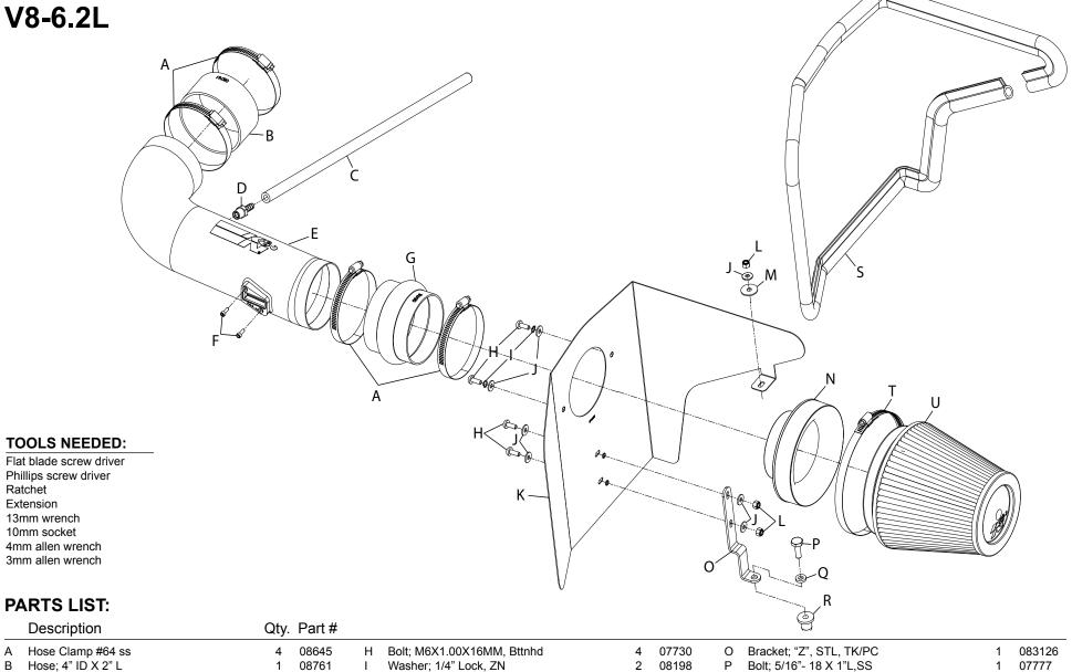
Vent; STRT, 5/16" Barbed, 1/4 NPT 08908 Heat Shield 074053 Insert; 5/16-18 X .600 OD X .730L 088002 Ε Intake Tube 27461 Nut; 6MM Nylock, Hexhead, SS 07512 Edge Trim (70") 102454 Bolt; M4 - 0.07 8MM, A/H CAP, SS 07733 Washer; 1"X.300X.100 21685 Hose Clamp # 104 08697 M Adaptor; #454 RF-1042 Hose; 4" ID X 3" L Hump 08418 27300 If you need any assistance please call 1-800-858-3333 to speak with a representative
