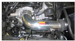
21. Install the K&N® intake tube assembly into the silicone hose at the filter adapter and then into the silicone hose at the throttle body and secure with the provided hose clamps.
