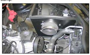
17. Install the silicone hose (08418) onto the filter adapter and secure with the provided hose clamp.
