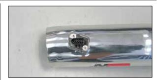
19. Install the mass air sensor into the K&N<sup>®</sup> intake tube and secure with the provided hardware.
