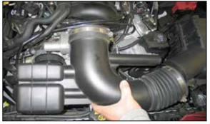
6. Remove the stock intake tube as shown.
