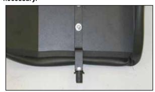
14. Install the inserted nut onto the heat shield mounting bracket using the provided hardware. Do not completely tighten at this time.
