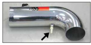
20. Install the provided 1/4npt fitting into the K&N® intake tube as shown.
