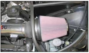
23. Install the K&N® air filter onto the filter adapter and secure with the provided hose clamp.
