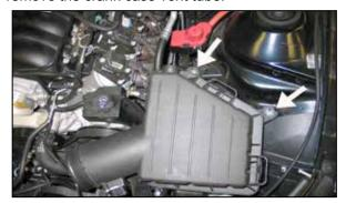
8. Remove the two air box retaining nuts shown.
