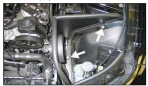
15. Install the heat shield assembly into the vehicle so the inserted nut goes into the air box mounting grommet hole and the tap goes onto the air box mounting stud. Secure the heat shield with the provided hardware.
