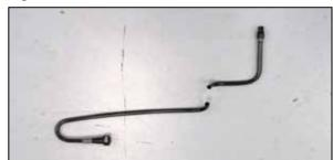
22a. On 2014 and later vehicles, it will be necessary to cut the crank case vent tube as shown. Then connect the cut section of tube to the oil filler cap. Attach the supplied hose to the trimmed section of crank case vent tube,
