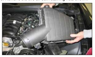
9. Lift up and remove the air box from the vehicle. NOTE: K&N Engineering, Inc., recommends that customers do not discard factory air intake.
