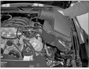
6. Remove the airbox assembly as shown.
