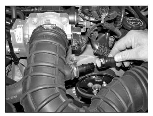
3. Rotate the green locking tab clockwise and then disconnect the crankcase breather hose from the intake tube.
