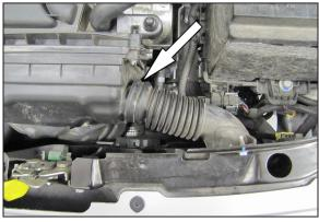
5. Disconnect the fresh air intake hose from the intake plenum.
