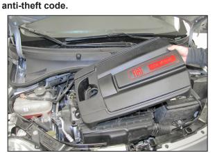
2. Lift up the engine cover and remove it from the engine.
