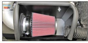
21. Install the K&N® air filter and secure with the provided hose clamp.
