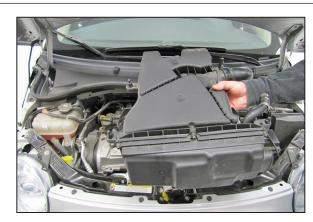
7. Lift up and remove the complete stock intake system from the engine.
