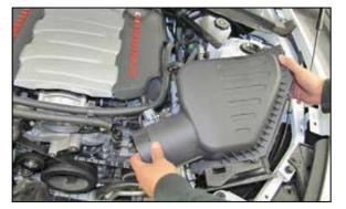
12. Lift up the air filter housing to dislodge it from the mounting grommets and then remove it from the vehicle.
