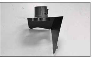
13. Install the K&N<sup>®</sup> mass air sensor housing into the heat shield and secure with the provided hardware.
