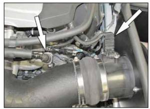
26. Connect the crank case vent hose to the quick disconnect fitting installed into the K&N<sup>®</sup> intake tube. Connect the mass air sensor electrical connection.
