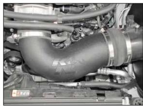
25. Install the K&N<sup>®</sup> intake tube into the hump coupler and then into the coupler at the throttle body, adjust the tube for best fit and then secure with the provided hose clamps.
