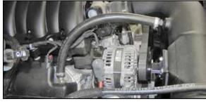
19. Install the provided crank case vent hose onto the valve cover port and onto the vent installed into the intake tube. Secure the hose with the provided hose clamps.
