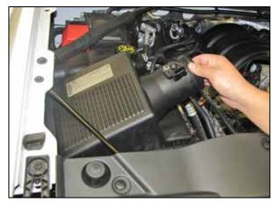
6. Lift up and remove the air filter housing from the vehicle.
