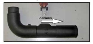
16. Install the mass air sensor assembly into the K&N® intake tube and secure with the provided hardware.
