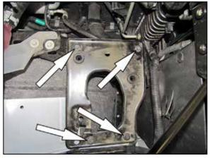
7. Remove the four bolts that secure the air filter housing mounting plate and then remove the plate from the vehicle.
