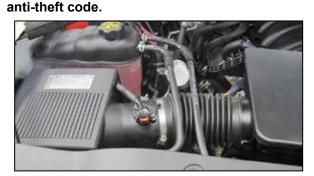
2. Disconnect the mass air sensor electrical connection and unhook the wiring harness from the air filter housing.
