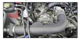
18. Install the K&N® intake tube into the hose at the filter adapter and then into the hose at the throttle body. Adjust the tube for best fit and then secure with the provided hose clamps.
