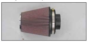
10. Install the filter adapter into the K&N® air filter and secure with the provided hose clamp
