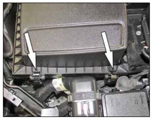
6. Release the two clips securing the upper air box to the lower air box.
