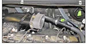
8. Install the provided hose coupler (08690) onto the turbo inlet and secure with the provided hose clamp.
