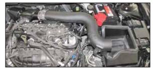
16. Install the K&N<sup>®</sup> intake tube into the coupling hose at the turbo inlet and align with the tube mounting bracket installed in step #8. Secure the tube with the provided hose clamp and hardware.
