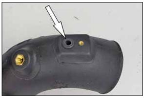
13. Install the provided grommet into the K&N<sup>®</sup> intake tube as shown.
