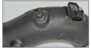
15. Install the quick disconnect fitting into the K&N<sup>®</sup> intake tube as shown.
