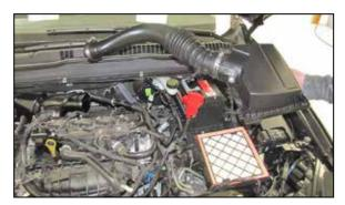
7. Lift up and remove the upper air box housing and intake tube from the vehicle. Remove the stock air filter.
