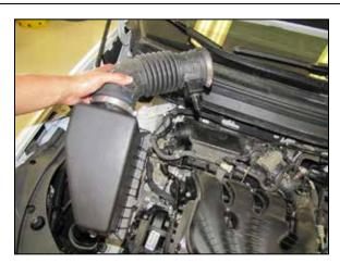
4. Loosen the hose clamp that secures the intake tube to the intake plenum. Disconnect the intake tube and then remove the complete intake system. NOTE: K&N Engineering, Inc., recommends that customers do not discard factory air intake.
