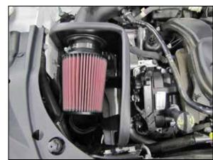
13. Install the K&N<sup>®</sup> air filter onto the intake tube and secure with the provided hose clamp.
