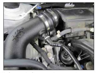
12. Connect the factory crank case vent hose to the quick connect fitting installed into the K&N<sup>®</sup> intake tube.
