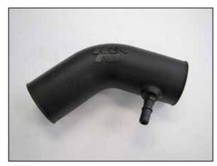
10. Install the vent fitting into the  $K\&N^{\otimes}$  intake tube as shown.
