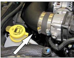
33. Reconnect the inlet air temperature sensor electrical connection.
