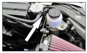
19. Install the heat shield bracket assembly onto the heat shield and radiator mount as shown. Secure the bracket with the factory bolt in step #9 and the hardware provided.
