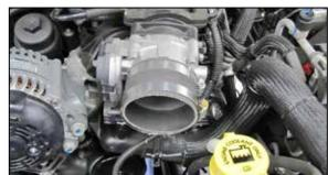
24. Install the provided silicone hose (08690) onto the throttle body and secure with the provided hose clamp.
