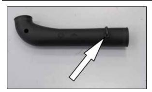
25. Install the 90°, ½" vent fitting into the K&N® intake tube as shown.
