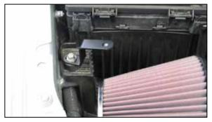
21. Install the provided bracket (083163) onto the rubber mounted stud using the provided hardware.
