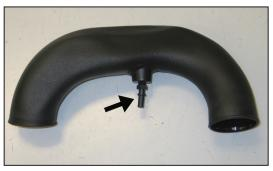
11. Install the provided crank case quick connect fitting into the K&N<sup>®</sup> intake tube as shown.
