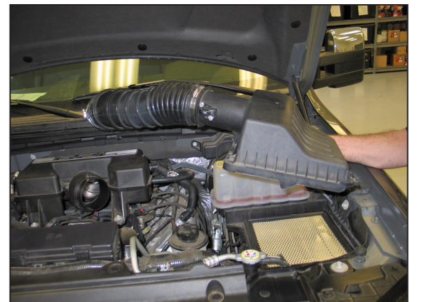
5. Remove the upper air box/intake hose assembly and air filter. NOTE: K&N Engineering, Inc., recommends that customers do not discard factory air intake.
