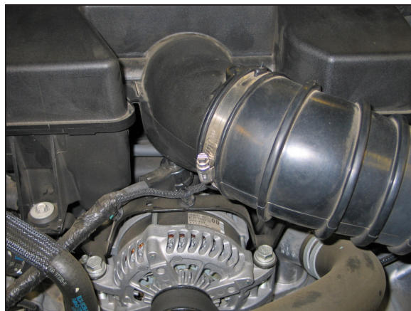
3. Loosen the hose clamp that secures the intake tube to the intake plenum.
