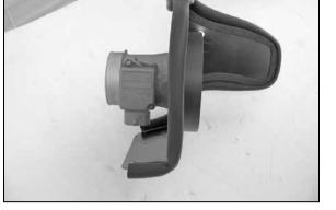
14. Assemble to mass air sensor to the heat shield and filter adaptor using the provided gaskets and hardware as shown.
