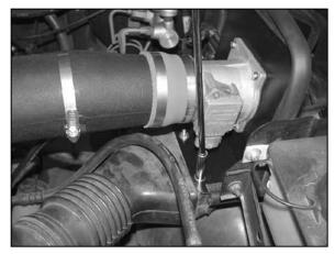
20. Mount the fresh air duct to the heat shield with the provided hardware.
