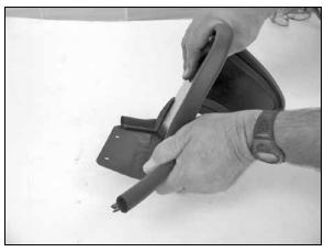
11. Install edge trim onto heat shield as shown. Trim if needed.
