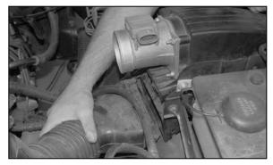
6. Remove the fresh air intake tube from the bottom of air box as shown.
