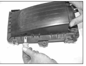
13. Twist the temp sensor counter clock wise to remove from the facotry airbox.
