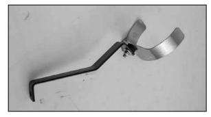
8a. On vehicles that do not come equipped with A/C, assemble the saddle bracket onto bracket (07165) as shown.
