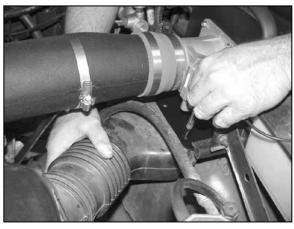
17. Install the mass air assembly onto the intake tube then line up the fresh air duct to the heat shield and mark the two holes with a marker.
