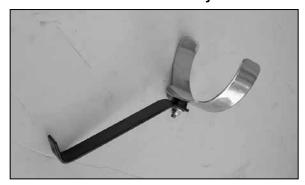
8. On vehicles that come equipped with A/C, assemble the saddle bracket onto bracket (07164) as shown.
