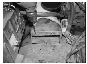
18. Remove the mass air assembly and drill two 1/4" holes were marked in the previous step.
