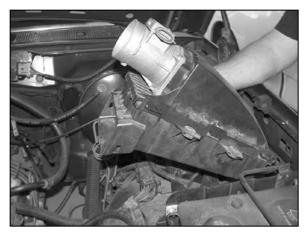
7. Remove the three bolts that secure the air box to the vehicle then remove air box from vehicle. **NOTE: K&N Engineering, Inc., recommends that customers do not discard factory air intake.**
