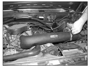
16. Install the new K&N<sup>®</sup> intake tube onto the throttle body, then secure the intake tube to the saddle bracket as shown.
