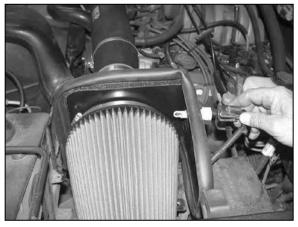
23. Install the temp sensor onto the heat shield then reconnect the electrical connection as shown.
