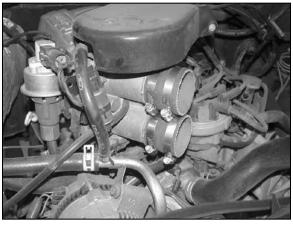
10. Secure the provided silicone hoses (08405) onto the throttle body with the provided hose clamps as shown.
