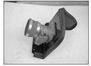
15. Install the silicone hose (08051) onto the mass air sensor with the provided hose clamps.
