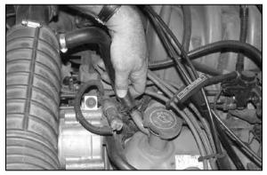
4. Loosen the hose clamp that secures the crank case vent to the calve cover then remove hose.
