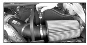
25. Install Air Filter onto intake tube as shown but do not tighten completely.
