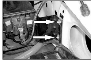
11. Remove the two bolts that retain the fuse box mounting bracket as shown.
