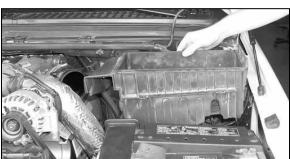
6. Then remove the stock airbox base from vehicle. NOTE: K&N Engineering, Inc., recommends that customers do not discard factory air intake.
