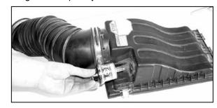
21. Remove air filter restriction gauge from stock airbox top.
