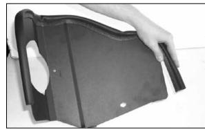
8. Apply the edge trim to the heat shield as shown. Trim if needed.
