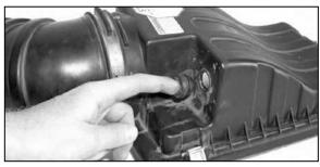
22. Remove restriction gauge grommet from stock airbox top.
