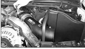
16. Install the K&N® intake tube onto intake manifold.
