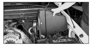
14. Install the heat shield and saddle bracket assembly as shown.
