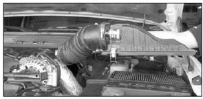
3. Loosen the hose clamp at the intake manifold. Release the clips from airbox top then remove complete upper intake.
