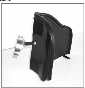
10. Install saddle bracket assembly onto heat shield as shown. Do not tighten completely.
