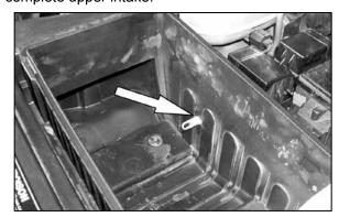
4. Remove the air temp sensor from the airbox.
