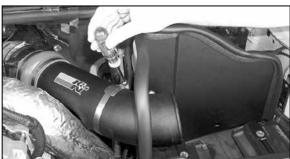
17. Install hose clamp onto saddle bracket and K&N® intake as shown.
