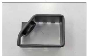
13. Install the provided edge trim onto the heat shield as shown.
