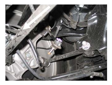
7. Remove the factory Anti-Sway Bar by removing the factory bushing brackets.
